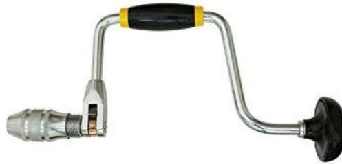
**Hand Drill:** For smaller diameter holes, smaller drills work better. Fiskars makes a plastic one that does fine for small projects, but their plastic gears wear down with use. Search garage sales for older metal ones or invest in a new one. Coordinating two hands doing different motions is a great challenge for the youngest. Some metal drills have a third handle, allowing a third hand to support.
